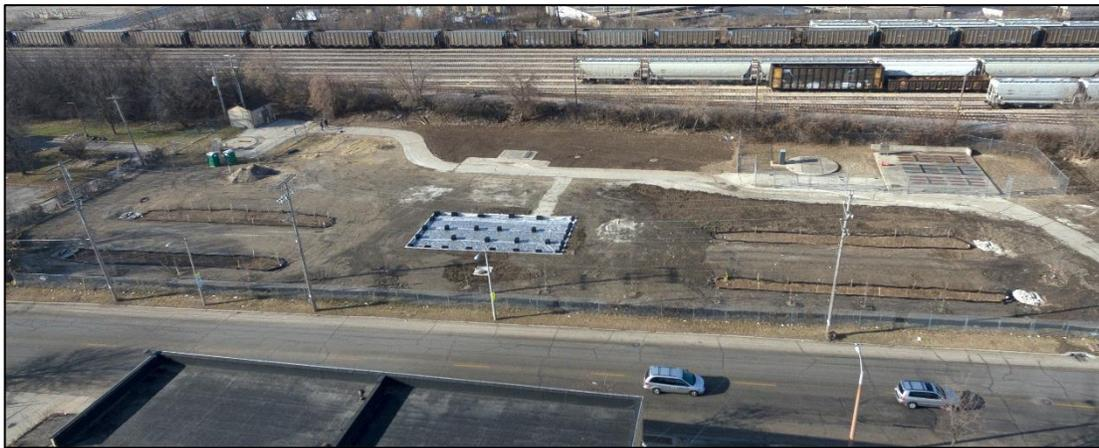
Drone photo of Green Tech Station from November 2018, looking west. Note the four bioswales are excavated and the cistern is installed (center)
