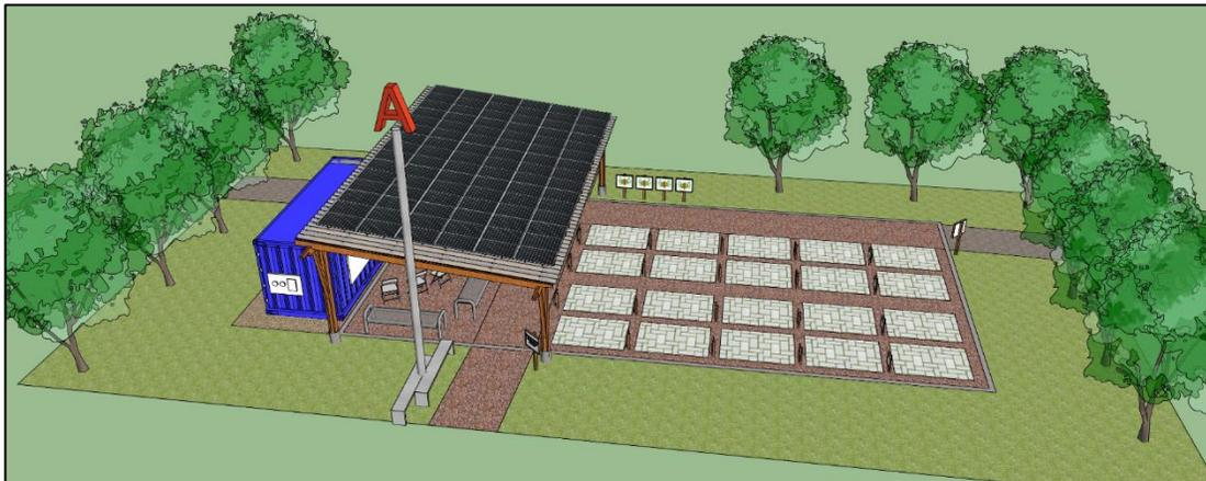
Rendering of the permeable pavement plaza space and shipping container storage area. This will be located on top of the cistern and feature test plots for demonstrating new green technologies.
